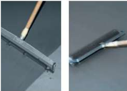
The cementitious floor levelling compound PCI Zarmtec® 140 must be applied evenly using a trowel and squeegas and then properly airrased with a spiked roller.
